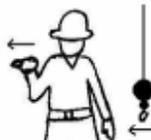
**TROLLEY TRAVEL** – With palm up, fingers closed and thumb pointing in direction of motion, hand is jerked horizontally in direction trolley is to travel.
